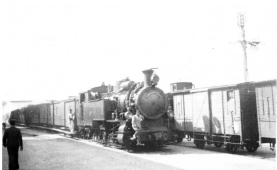
11:20 D. H. P. (1.05m. gauge) 0-10-0T loco no. 301 on train at Beirut Harbour Station. (S.L.M. Winterthur 1924). 4th. April 1939. Photo: R. A. Wright.
