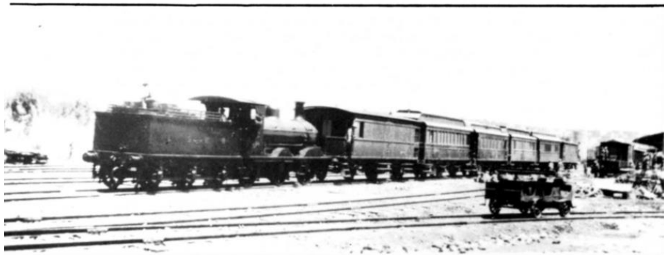
Not Mesopotamia, but an LSWR Jumbo 0-6-0 on a train (General Allenby's train ?) at Jerusalem. N. B. Tender bears "L. S. W. R. markings", no "W. D. " number. Motorised draisine in foreground Photo: Ron Garraway.
