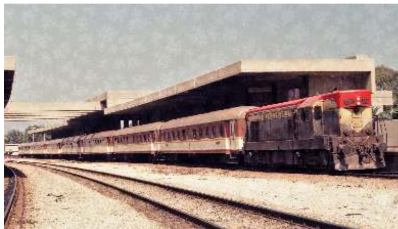
• Picture 5: train no. 24 (09h00 Tel Aviv Merkaz – Haifa Merkaz) hauled by ex-ESR EMD G12 no. 127 ready to depart Haifa Bat-Galim on 17.8.1987. This loco was rarely used to haul passenger trains. Note the first coach is a refurbished Metalka (Boris Kidri?) coach used as a reserved seat coach replacing a Mk2c.
