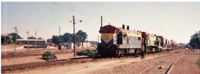
• 4,000-ton Train No. 856 (10:40 Dimona to Ashdod) arriving at Lod New Loop on a sunny afternoon in the summer of 1980. The train was double-headed by G26CW No. 604 and G12 No. 112 up to Na'an from where it was triple-headed on to Lod by G12 No. 116 to assist in coping with the 1.2% incline. (photo: Harel Even)
