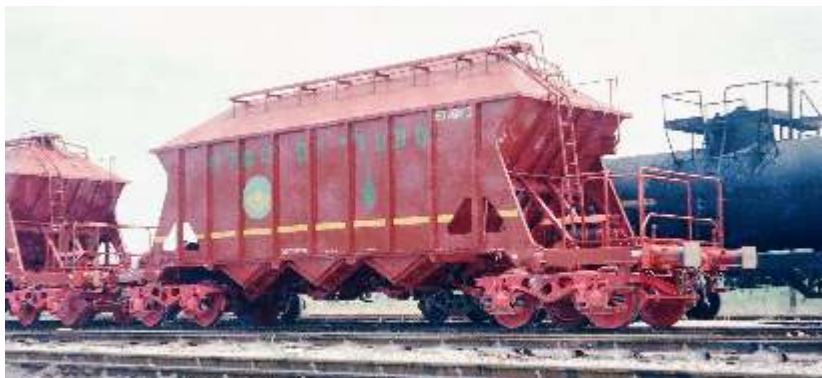
• Brand-new Metal wagon No. 60 839 ? (Chaf) in Haifa East yard in the summer of 1980 already carrying a Dead Sea Works logo as well as the ISR logo. It was renumbered later as 65 839 ? (Chaf) with permitted payload raised to 65 tons. The majority of this type of wagon are currently stabled at Oron (photo: Harel Even)
