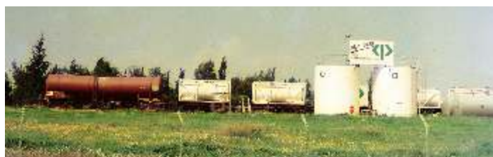
77,000 litre ex-white oil bogie tank wagon no. 77 015 ? (Daled) loaded with Ammonia and 50-ton bogie flat wagon no. 50 028 ? (Tet) loaded with ISO Containers unloading at the terminal in Kiryat Gat. (photo: Harel Even)
