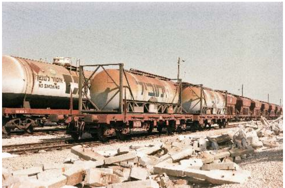
• La Brugeoise 60-ton bogie flats loaded with empty 30 feet ISO containers for Caustic Soda on 19.4.1986 en-route southbound at Haifa East yard. Behind are loaded Gaz tanks from the refineries to Gililot coupled to empty hoppers from Haifa Chemicals southbound. (photo: Harel Even)
