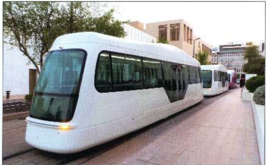
• The entire fleet of the new tram line in the centre of Doha. The three trams use LPG as fuel but will in the future possibly work with hydrogen. 5 September 2018. Foto: TIG/m."
