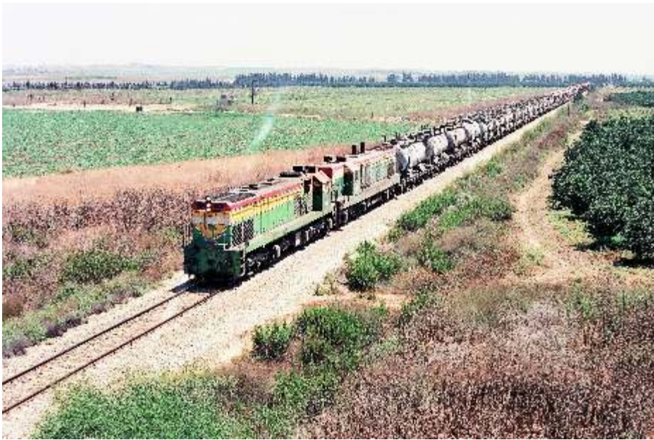
• EMD G26CW No. 601 and Ex-ESR G16 No. 161 double-heading a 43-wagon train no. 860 from Dimona loaded with phosphoric acid, phosphate and potash for Ashdod Port on 9.8.1988 south of Ashkelon. The three leading phosphoric acid tanks were from the first series manufactured in 1971 (photo: Harel Even)
