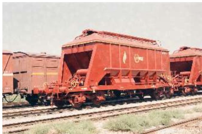
• Brand-new Arbel wagon No. 60 717 ? (Tzadi) in Haifa East yard after arrival from Vulcan Handassa works in Haifa bay in 24.6.1987 already carrying a Keter Tovala logo alongside the Negev Phosphate logo. The works used to be connected by a private siding to the Haifa – Bezet main line near Kishon block post. The wagon was renumbered later as 65 717 ? (Tzadi) with permitted payload raised to 65 tons (photo: Harel Even)
