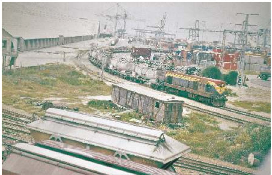
• Ex-ESR EMD G8 No. 251 shunting empty phosphoric acid tanks and flats loaded with steel coils from the docks at Ashdod Port to Ashdod Yard on 29.3.1988. The first three wagons were manufactured by Wagon Union seven years earlier for ISR but at the time the picture was taken already belonged to ICL. (photo: Harel Even)
