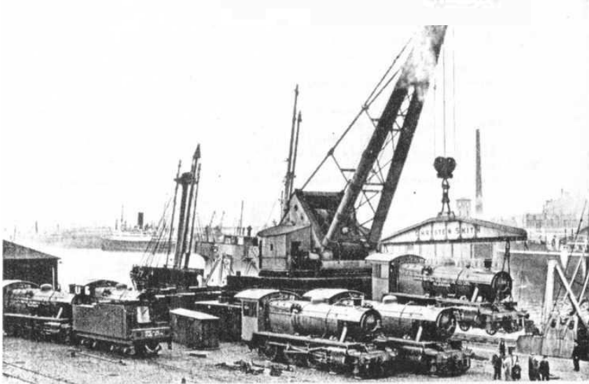
Completely assembled 4-6-0 locomotive built by the North British Locomotive Co. Ltd., for the Palestine, Railways bring shipped from the Clyde on one of Christen Smith's "Belships"
