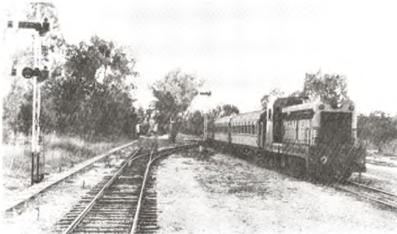
A Belgian-built Bo-Bo at Wadi Surar about 1960 with a train for Jerusalem, made up of ex-PR coaches. The station building is just out of picture to the right. At left is the siding leading into the military camp originally built by the British in World War 2. This siding seems to have been laid on the formation of the Turkish WW1 line to Beersheba (the 'Egyptian branch'). Note the covered van just visible in the distance. The posts of two of the semaphore signals can still be seen here, as well as rusted lengths of the siding, but connections to the main line are cut.
