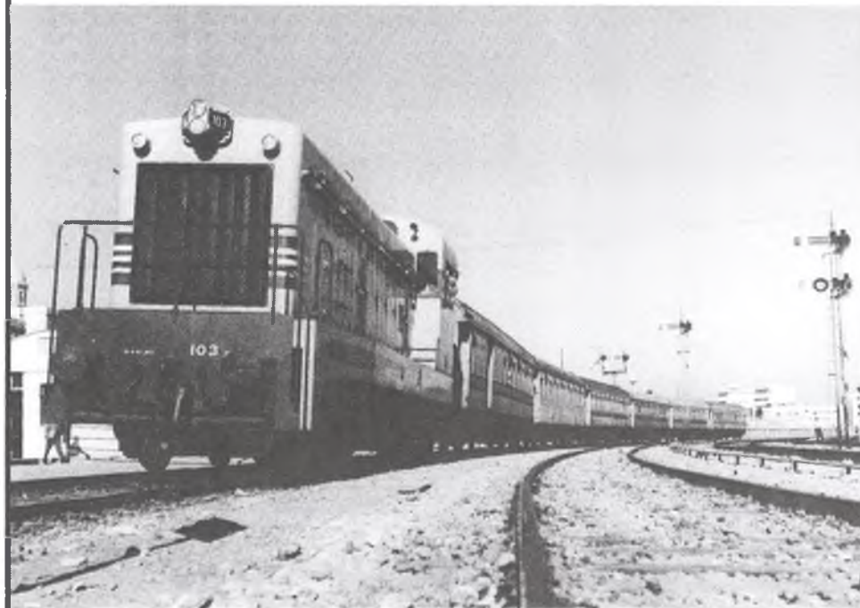
27:1 Quite a well known picture: IR SAFB Bo-Bo 103 entering Haifa Mizrach from Haifa Merkaz, ca 1958 with a 6 coach train of former PR stock. (Photo: Israel Govt. Press Office: ref 11843, File 13.2.1) Note the signals - only recently removed and the American style number on the bonnet light. Why on earth is that signal in the background "off"?
