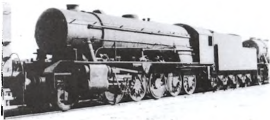
27:3. WD 2-10-0 No. 73674 (NBL 25460/44) at 169 Railway Workshops, Royal Engineers, Suez, 9th. Jan. 1945. (Photo: Len Redshaw.)
