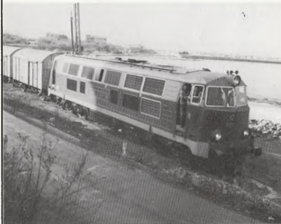
28:1 SYMBOLIC OF MOVES FOR FUTURE REINSTATEMENT OF REGULAR TRAFFIC: CEL Polish (Cegielski) built Co-Co diesel loco 1203 of 1977 at Dbaiye, about 8km north of Beirut, on a freight train. The train is standing just before a level crossing which is being dug out from the mud!
