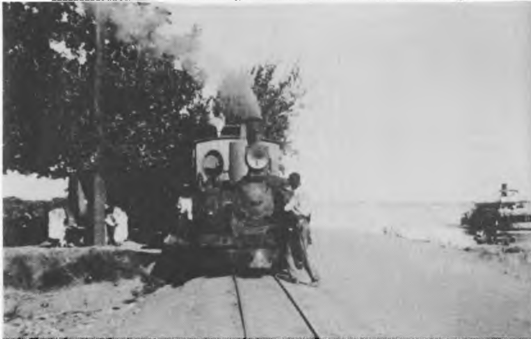
30: 12 The Khartoum Steam Tram. No further details available on original print, but the loco appears to be a Krauss 60cm. gauge tank. (Photo: The Tank Museum, Bovington.)
