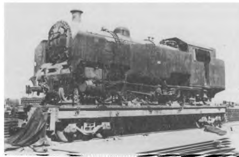
No: 20 WD 143, one of 6 metre-gauge 4-6-4T's originally built for Malaya but diverted to the Qena-Safage Railway in Upper Egypt, in store at Suez Royal Engineers Workshops. ca. Jan. 1947. (Photo: D. S. Currie.)
