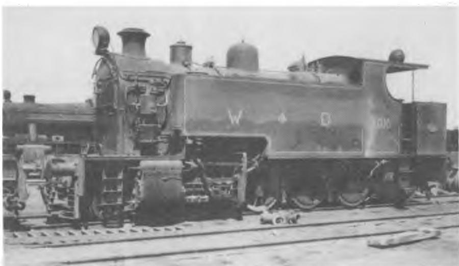
33:14: W.D. 2-8-2T No. 1015 at Suez, April 1948. Built by Hudswell Clarke 1942, and used briefly on the HBT Railway. Seen under overhaul or storage, minus coupling rods.
