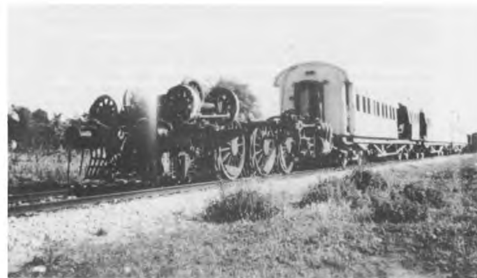
33.6. Result of sabotage near Lydda, 1947. Remains of a 4-6-0 (the bogie now on top of the frames) and some damaged PR coaches. (Photo: John Lee).
