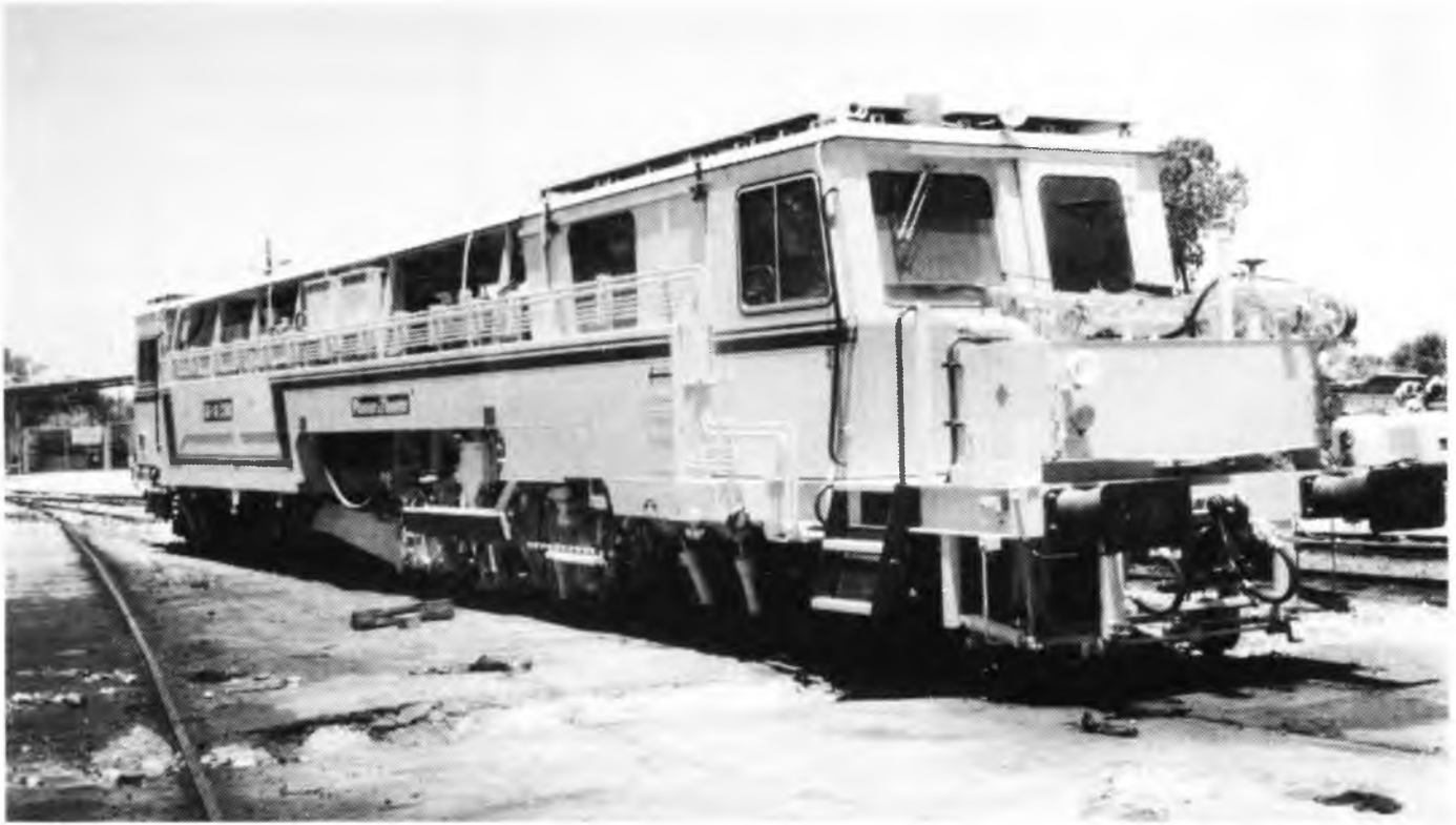
New I.R. Plasser & Theurer Tamper No. 2 (Type 09-16CSM) at Haifa PW-equipment workshops, 31/7/98. (Photo: Chen Melling.)
