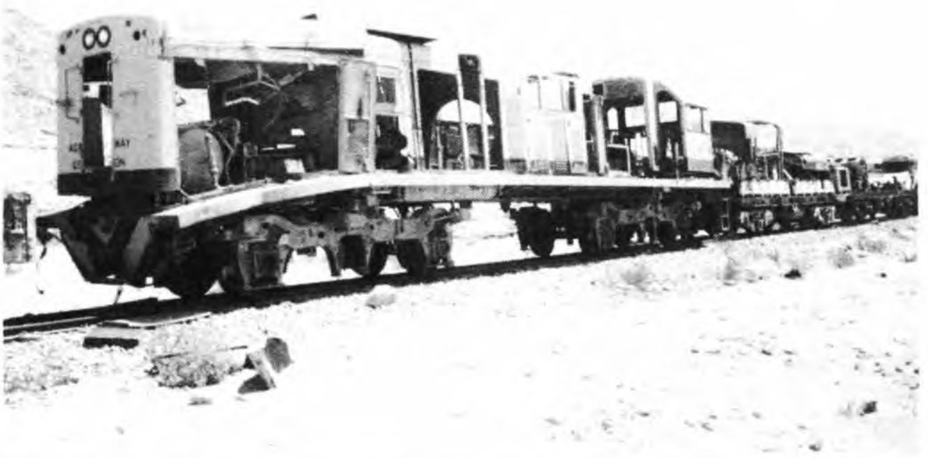
42:22. The harsh reality of modern operations on the Hedjaz Railway and its offshoot to Aqaba. GE U20C loco No. 312 (built 1979) stands, badly damaged, at Aqaba depot - a write-off by the look of it.
