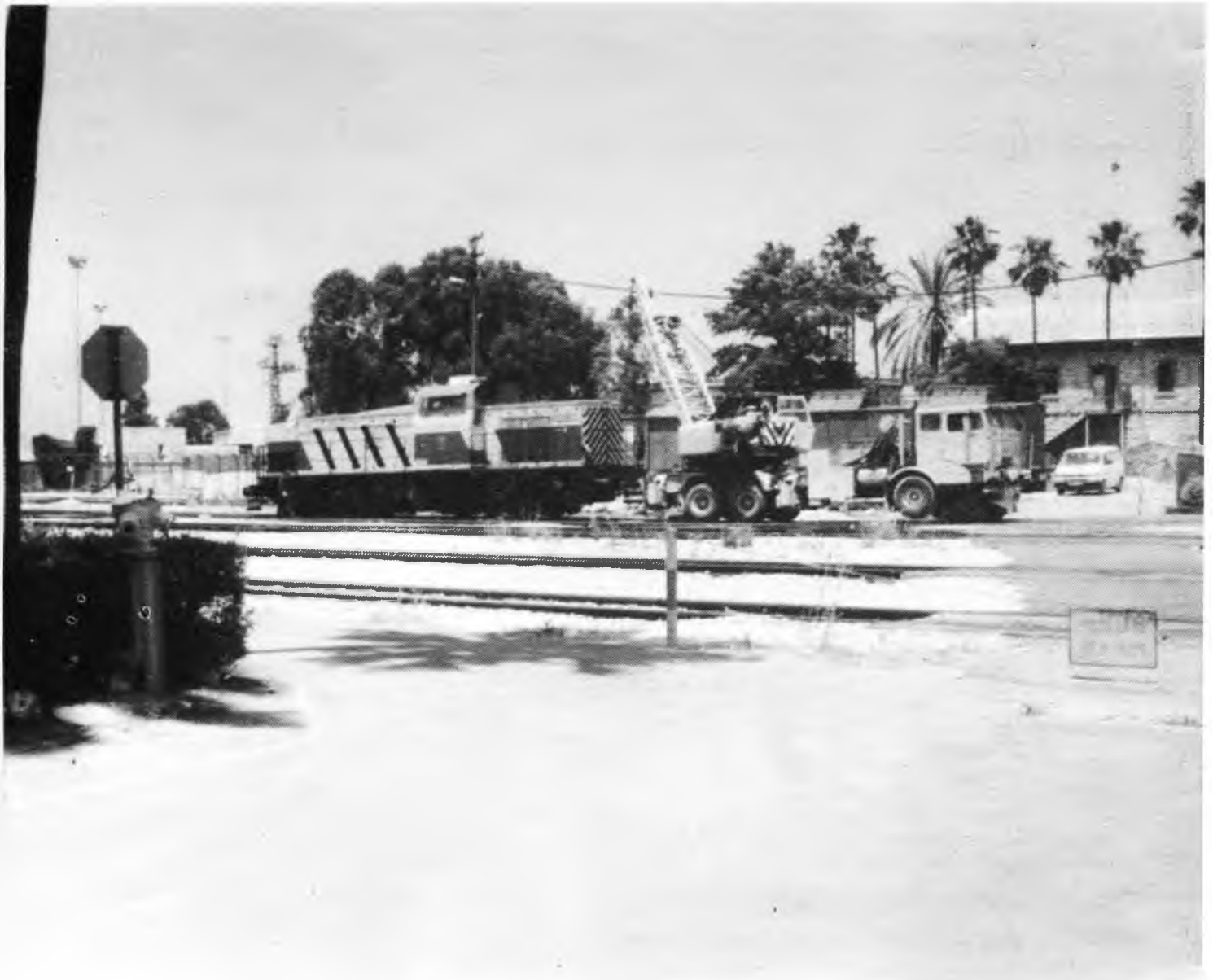
Bo-Bo T44 being rerailed at Halfa East yard, 28/6/98, after a minor derailment. (Photo: Theo Pelz.)
