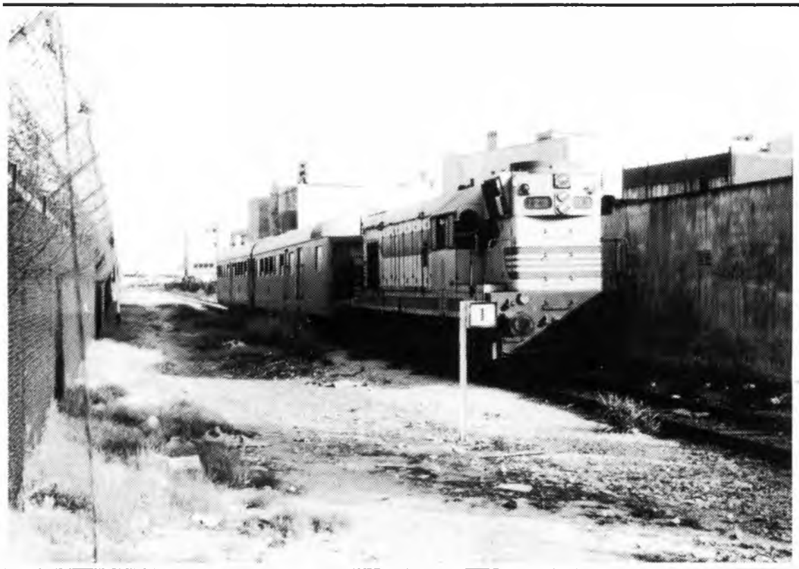
46:3. (Photo 2). Haifa as it was: G12 Bo-Bo No. 123 at Km. 1 on 20/5/70, hauling two former Esslingen trailers on an overgrown single track. (Photo: R.A. Bowen.)
