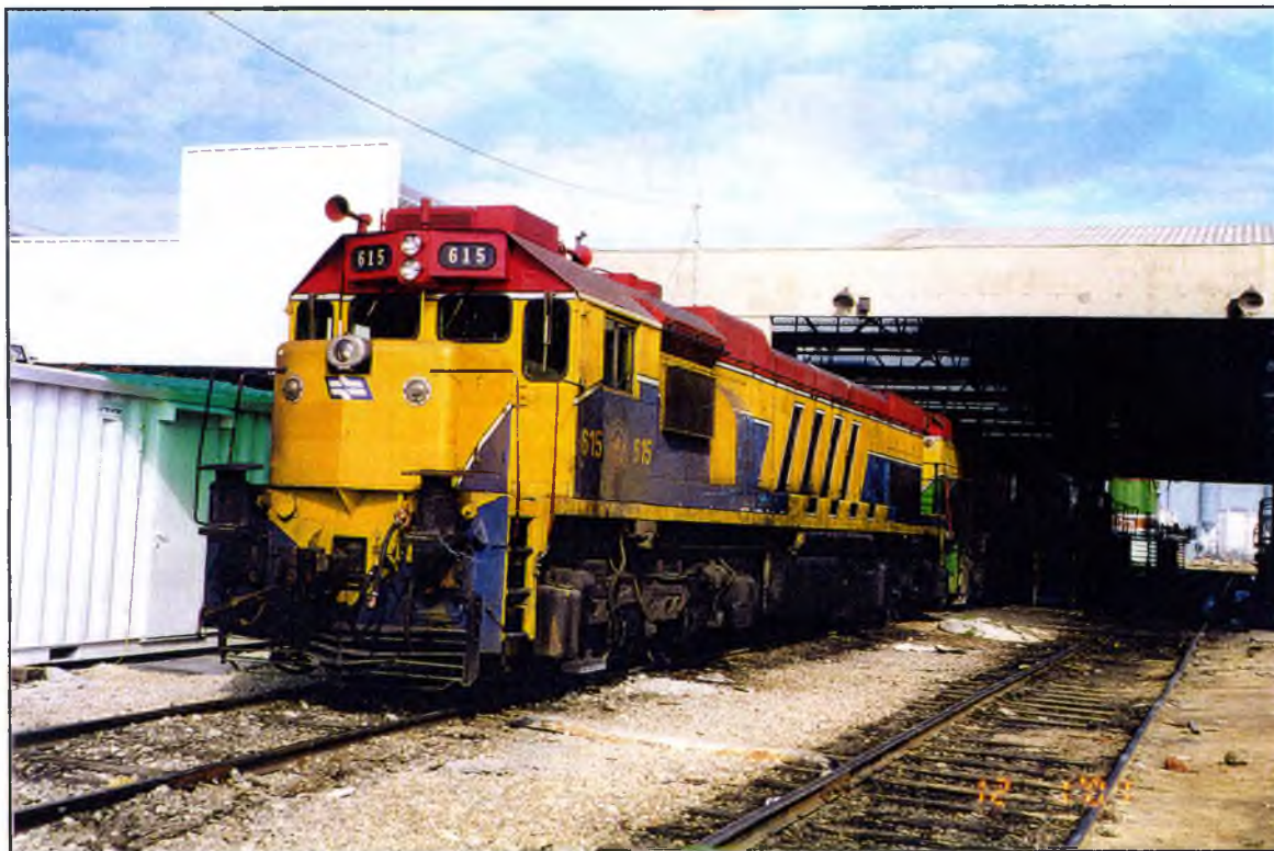
A Gm-EMD GT26W #615 at Lod old depot. The new one can be partially seen on the left. To be noticed is the ability of the loco to operate both with buffers and screw couplers and with automatic couplers only. Here the second option is applied with buffers lifted!
