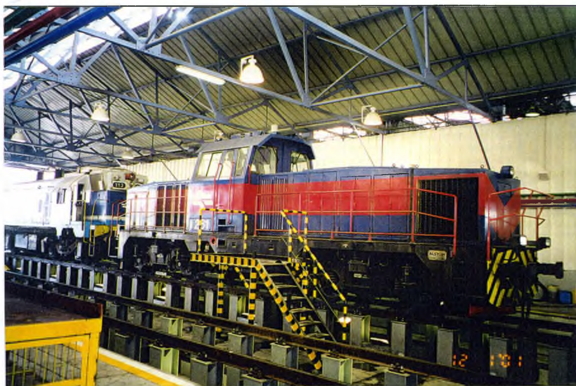
2 Generations at the new Lod Locos Depot: a veteran GM EMD G-12 #113 behind an Alstom series 900 new diesel - electric shunter powered by an MTU motor, identical to the shunters sold to SBB (except the airconditioning). Both above photos: Aharon Gazit
