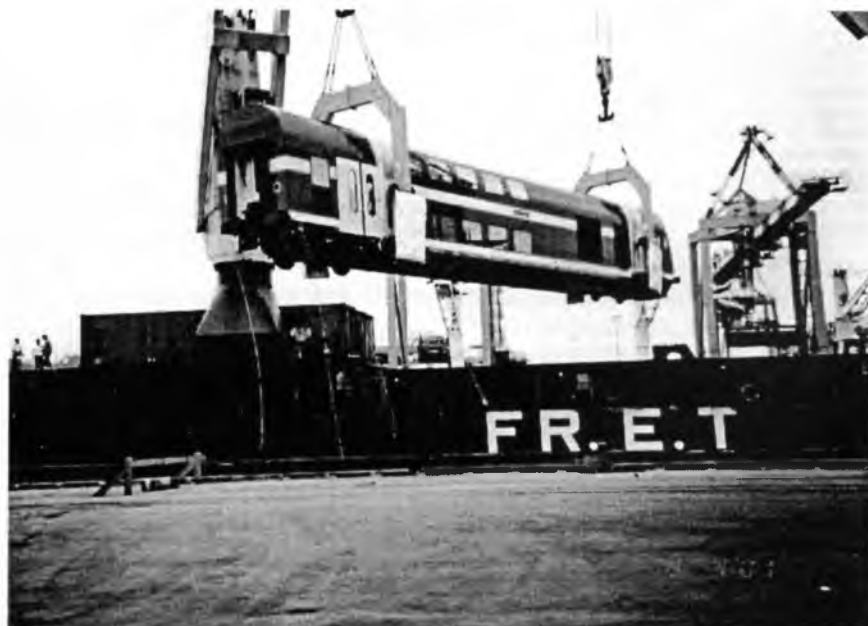
A Driving Trailer from Bombardier at Görlitz being unloaded at Ashdod Port. (Photo: Aharon Gazit.)
