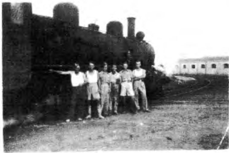
"A grubby Baldwin 4-6-0 at the original Tel Aviv (South) station in 1936. Not the best of snapshots by any means, but it does show the severe curvature of the lines here - an inheritance from the metre gauge J&J. In the background the line curves round to the left on its way down to Jaffa. Zev Gelblum stands third from right. (Paul Cotterell: IRM Archives.)"
