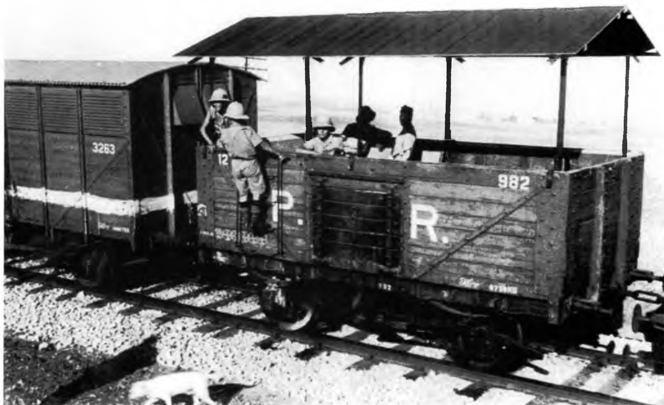
2. PR 12-ton high-sided open wagon No. 982 (ex-GWR?) bullet-proofed by addition of concrete lining and floor, in use with the breakdown train.
