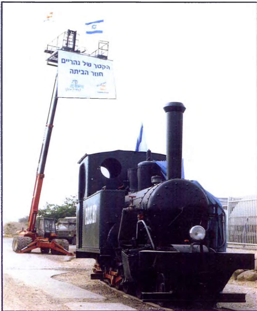
War Department Light Railway 60cm gauge Hunslet 4-6-0T, Palestine Electric Corporation H7, has been rebuilt at Kibbutz En Shemer and fitted with new parts for those that had gone missing (including dummy boiler, chimney and steam dome). It has a diesel engine hidden in the boiler shell and now operates again over a short length of track with five small tip wagons at 'Old Geshet' in the Jordan Valley, near Naharayim where it worked in building the Rutenberg Hydro-Electric Power Station over seventy years ago. It is seen at 'Old Geshet' ready for the recommissioning ceremony on 11th May 2004. The banner in the background reads "The Naharayim loco comes home". (Photo: Paul Cotterell)
