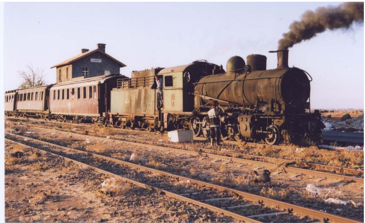
73:1. At Gasim, between Dera'a and Neesib, 5km. south of Dera'a, Syrian Hartmann centenarian 2-8-0 No. 91 built 1906 prepares to take special train along the Bosra branch in October 2005. (Photo: Robert Humm).
